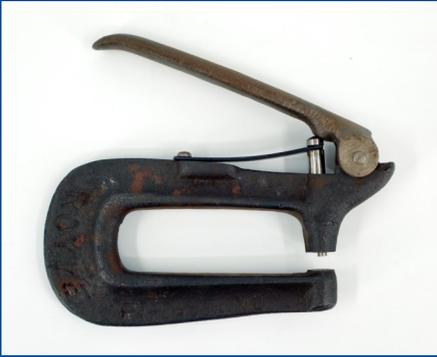
This hole punch is not just your average office tool. This punch, made by Royle & Sons, was used in the creation of jacquard cards. Sometimes when cards were run through the punch machine there would be a missed hole or one that was not fully cut. With this small tool, errors could be manually corrected. Why is this so important? The placement of the holes on the cards is what directs the machines to create the patterns in the fabric.
